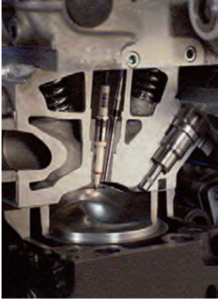
Figure 5.23 Cylinder pressure sensor mounted in the engine
