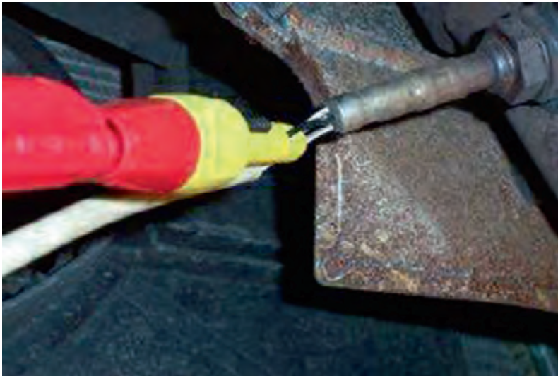
Figure 4.23 Titania knock sensor in position
