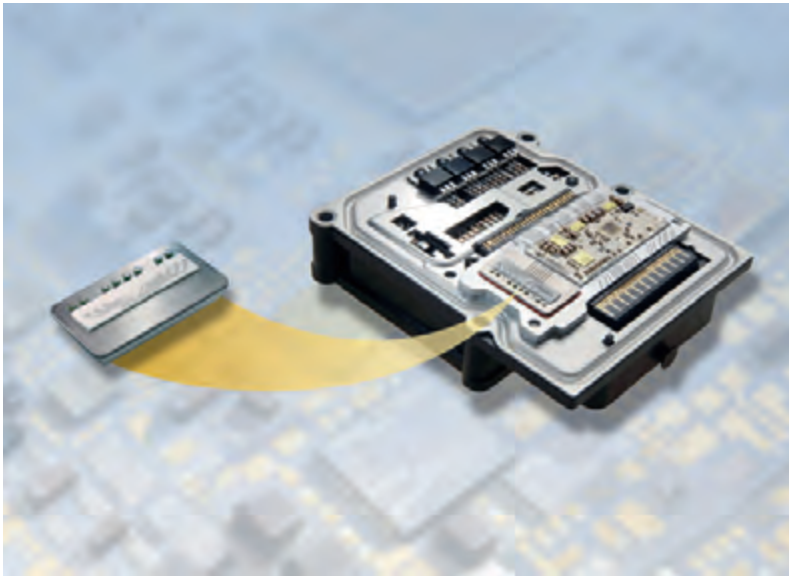
Figure 4.36 Yaw rate and acceleration sensor integrated into an electric stability program (ESP) control unit (Source: Bosch Media)
