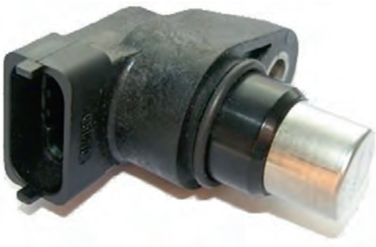
Figure 4.18 Hall effect ABS or CAS sensor
