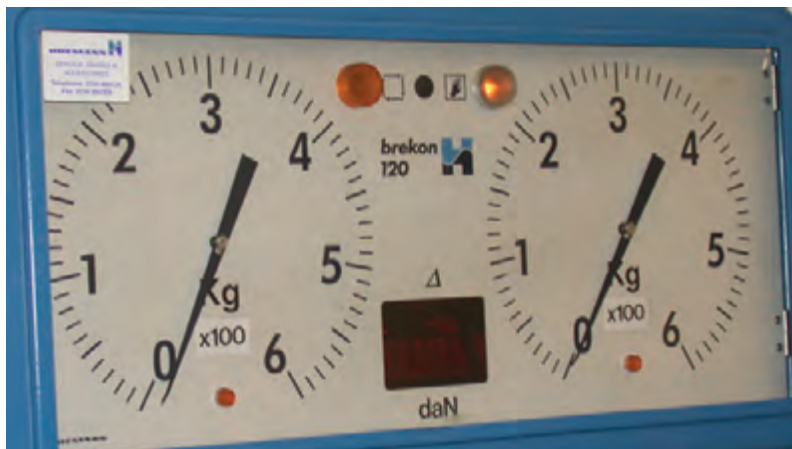
Figure 7.6 Gauges on a rolling road brake tester
