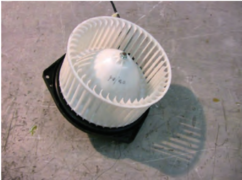
Figure 8.73 Blower motor and fan
