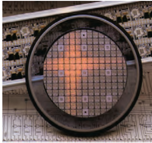
Figure 8.2 Silicon wafer used in the construction of integrated circuits
