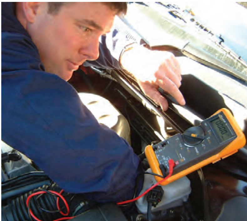
Figure 8.78 Circuit voltage testing
