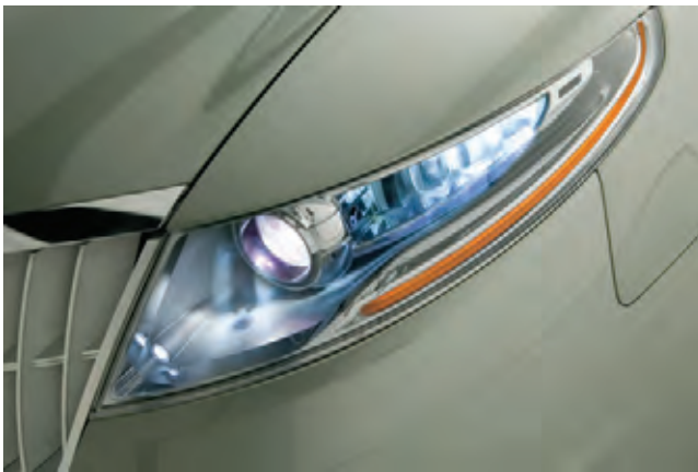
Figure 8.27 Adaptive lighting using LEDs
