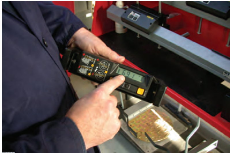
Figure 7.26 Laser alignment systems give digital readouts
