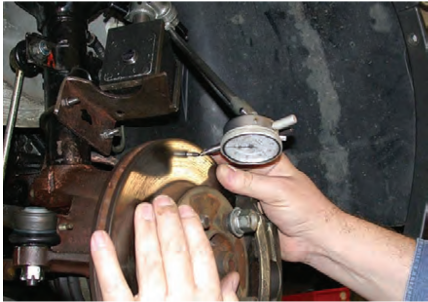
Figure 7.7 Checking for brake disc run out with a dial gauge
