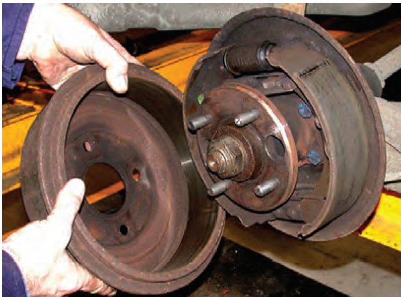
Figure 7.4 Drum brakes showing the shoes and wheel cylinder
