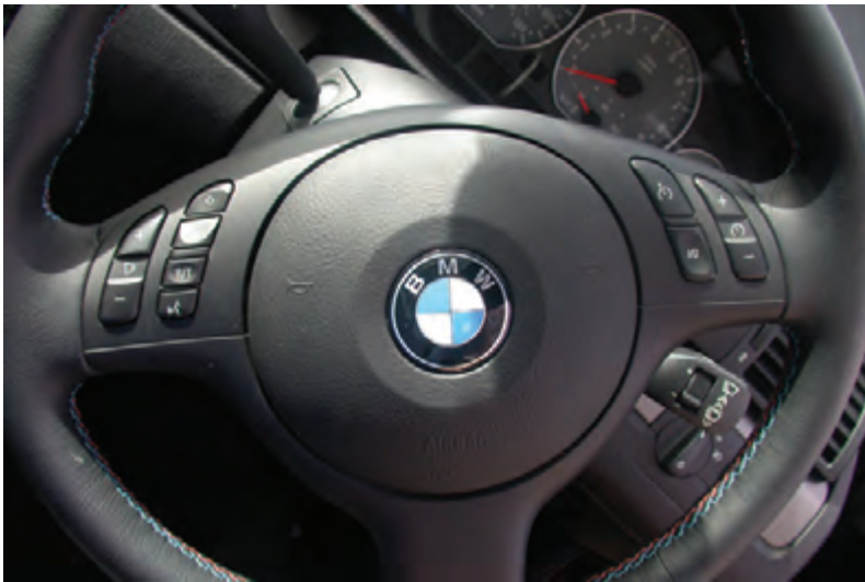
Figure 8.86 The driver's airbag is incorporated into the steering wheel
