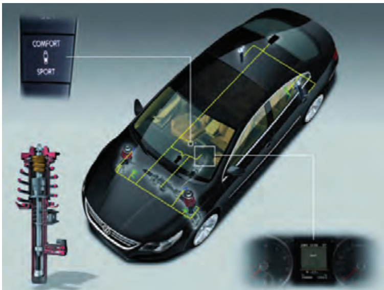
Figure 7.37 Active suspension also allows adjustments; in this case, between sport and comfort settings(Source: Volkswagen Media)
