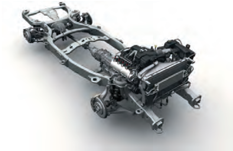
Figure 9.6 4 WD transmission layout (Source: Ford Media)
