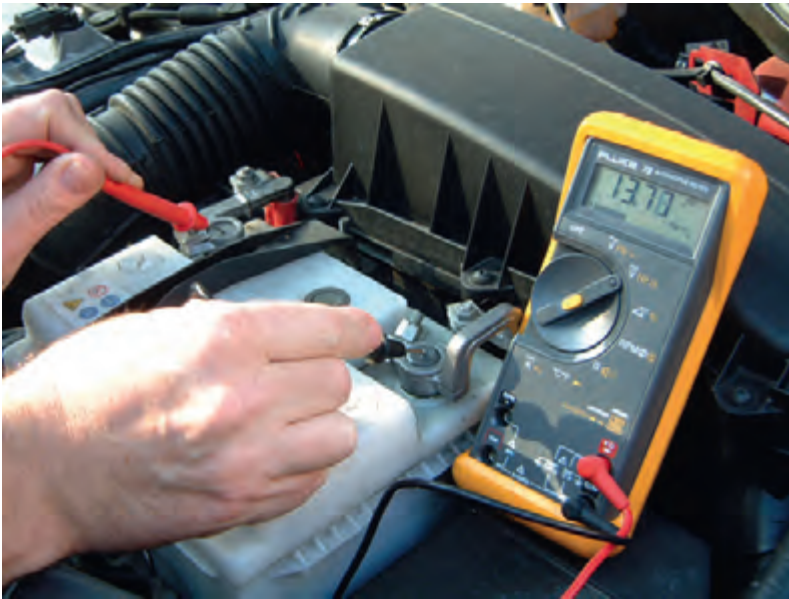
Figure 6.80 Checking battery voltage. In this case, the engine had just been switched off so the reading shows a 'surface charge'
