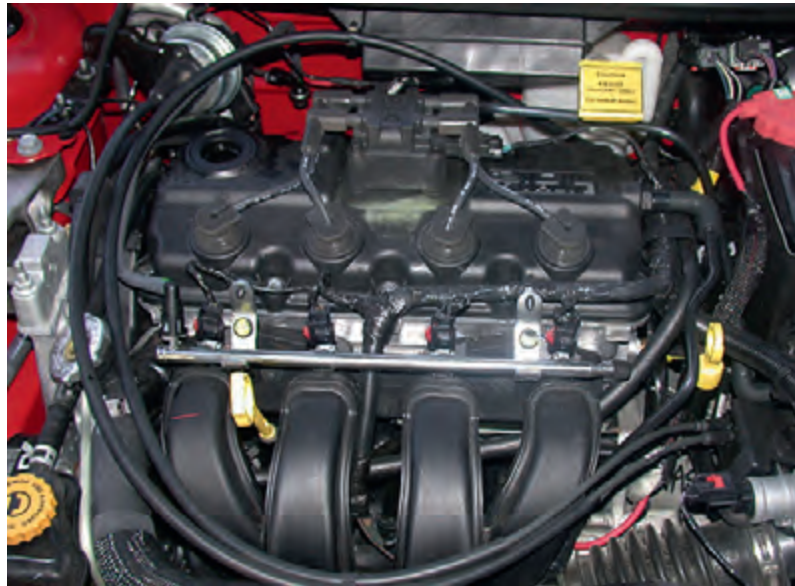
Figure 6.25 DIS coil on a four-cylinder engine
