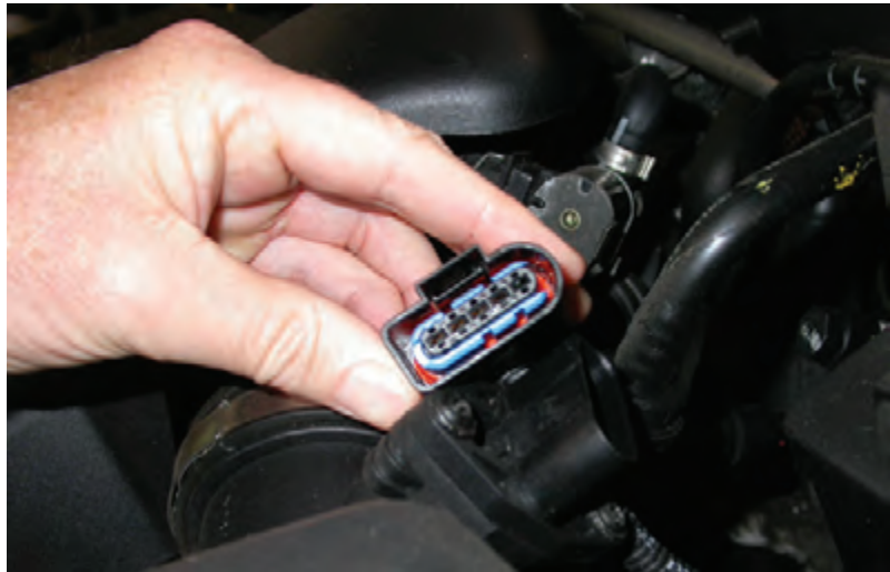
Figure 6.65 Airflow meter under test
