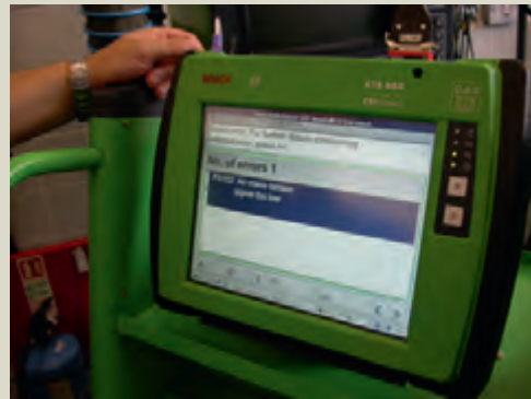
Figure 3.14 Take a readout from the control unit memory (DTC display)
