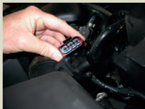
Figure 3.15 Airflow sensor connection
