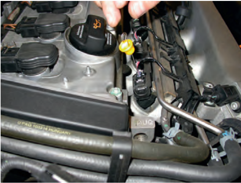
Figure 2.12 Test the voltage by back probing a connector with care
